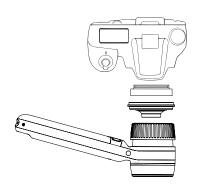
The HEINE SLR | SLM Camera Adapter flow can be used with a DSLR or DSLM camera with an existing fixed focal length lens that has an M52 or M49 connection thread. It is suitable for use with the HEINE DELTA 30 PRO and the HEINE DELTA 30. Any reference to the DELTA 30 PRO in this document is a reference to both instruments.
