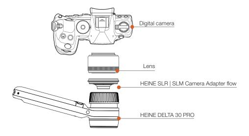
Screw the camera adapter onto the lens' filter thread connection.
